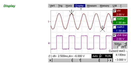
*Composition* The oscilloscope display is divided into 4 functional zones.
