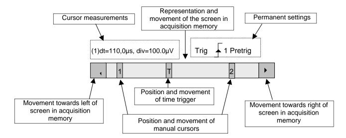
Each element in the bargraph can be moved with the stylus.
