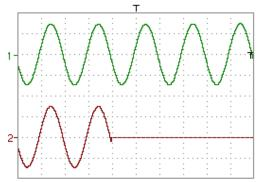
The result of math2 is equal to ch1 as long as **t** is less than four horizontal divisions (t-divh(4) > 0).
