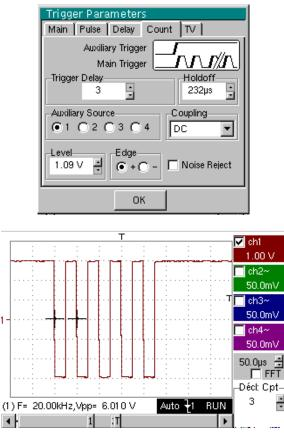
The trigger is set on the trailing edge.
