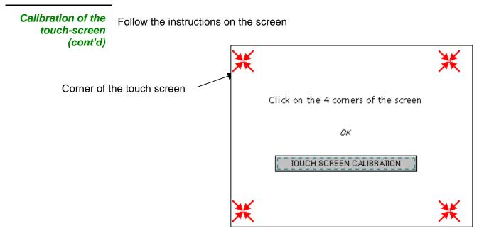
Use the stylus to point at the centre of the 4 patterns displayed on the screen. Validation of the input is indicated by modification of the pattern.
