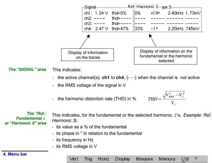
The same menu toolbar is used as in "Oscilloscope" mode; some menus are adapted to the "Harmonic Analysis" mode and the others are not active.
