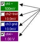
Using the stylus, display of: the parameters of the traces in the same color as the trace: validity, coupling, bandwidth limit, sensitivity
