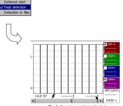
The fault capture mode is selected: the screen is divided into 10 sections.
