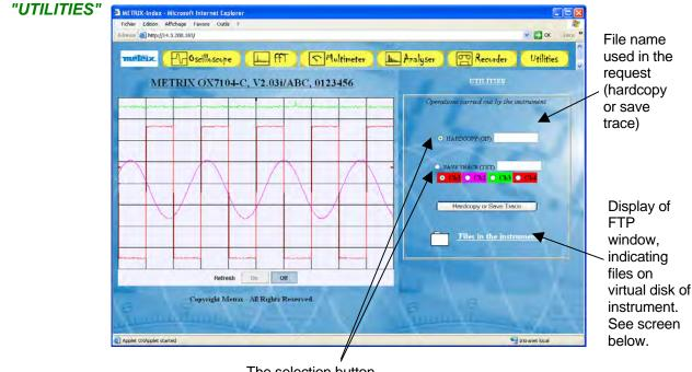
The selection button determines the action: - launching of screen copy or
