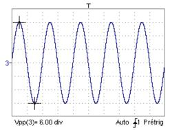
The trace obtained is a sine-curve produced using the predefined function "sin()". The amplitude is 6 divisions.
