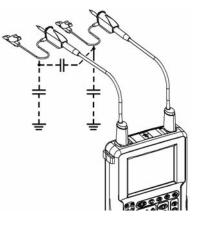
It is essential, given the stray capacitances, to connect properly the reference conductors for each probe. These conductors must be connected preferably to the cold points, to prevent transmission of noise by the stray capacitance between modes.
