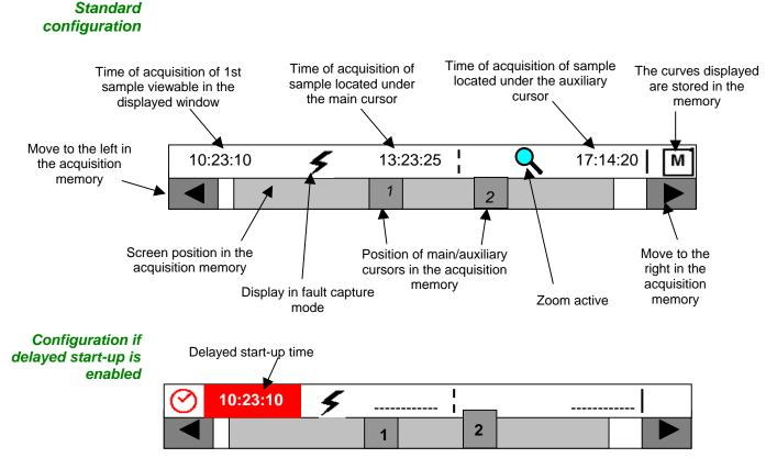
When the acquisition starts, the display returns to its standard configuration.
