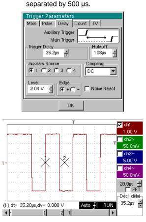
The trigger is active after the end of the delay (35.2  $\mu$ s) on the first leading edge. The Holdoff stabilizes the signal by disabling the trigger for 108  $\mu$ s.
