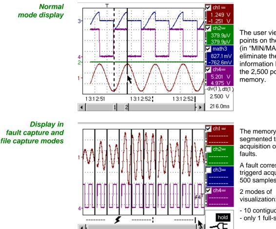
The user views 500 points on the screen (in "MIN/MAX" mode) to eliminate the risk of information loss involving the 2,500 points in the
