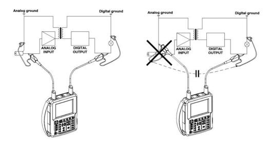
The noise of the digital ground is transmitted to the analog entry by the stray capacity.
