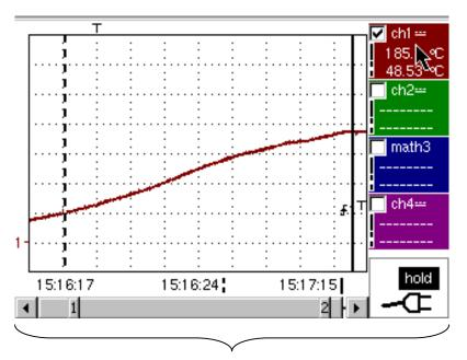
This acquisition shows the heating dynamic of the soldering iron.
