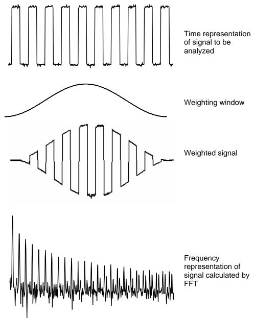
The finite duration of the study interval results in a convolution in the signal frequency domain with a function sinx/x.
