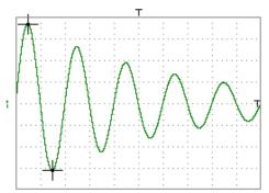
"sin (pi\*t/divh(1))" can be used to modify the number of periods. "exp (-t/divh(6))" can be used to modify the level of attenuation.
