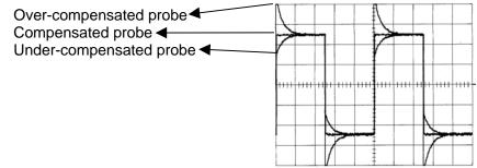
Adjust the screw on the **PROBIX HX0030** probe to adjust the compensation.
